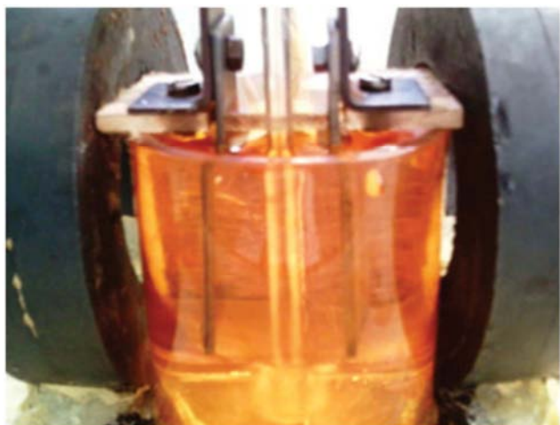
Figure 3. The apparatus of EC with MF magnets placed for the treatment of MO [29].
