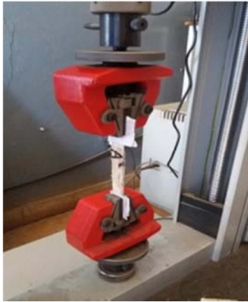
Figure 6. Test specimens and ASTM (M500-50KN) for tensile testing.
