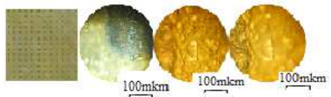
Fig. 2. a) Optical image of the soft magnetic substrate: the distance between the squares centers is 1.65 mm. Squares side is 0.35-0.4 mm. b) the middle of the step is 20 μm; c) bottom of the step; d) top of the step.
