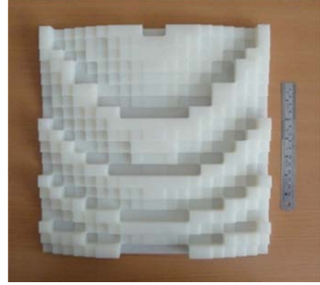
Figure 4. Fabricated nonuniform dielectric transmit array antenna.
