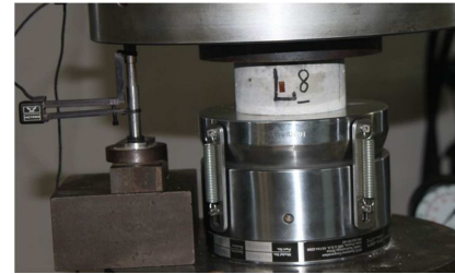
Figure 2. Uniaxial compression of a specimen.
