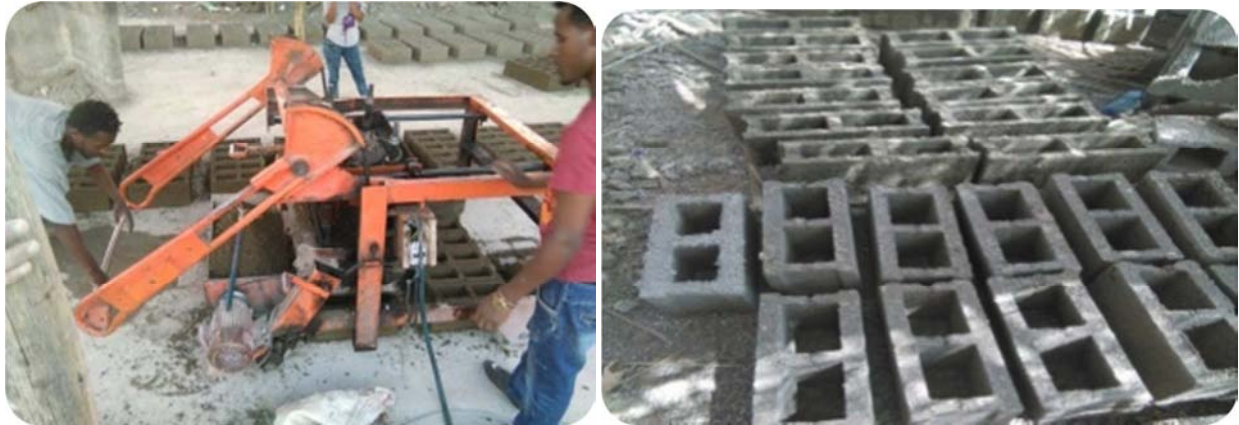
Figure 7. Production process of Papercrete hollow block.
