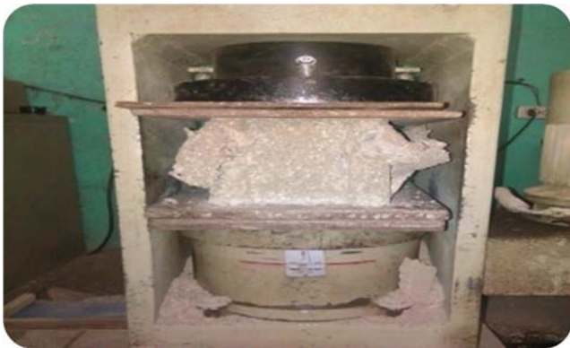
Figure 9. Papercrete hollow block under compression.
