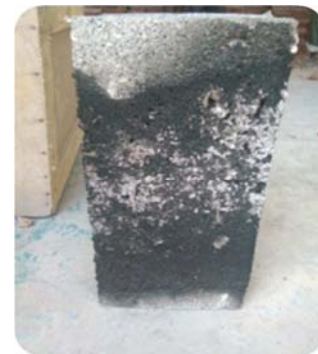
Figure 12. Papercrete hollow blocks after fire resistance test.
