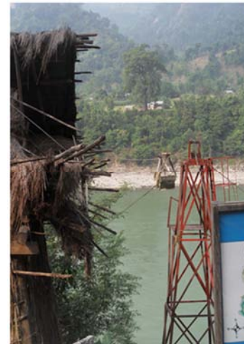
Figure 4. Cableway in Chatra for measuring of flow and suspended sediment.
