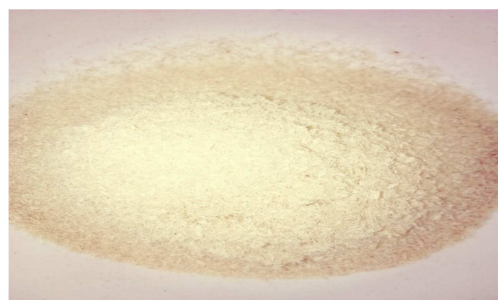
Figure 3. Sodium hydroxide modified Kenaf fiber.
