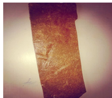
Figure 4. Fabricated Kenaf fiber-PE composite.
