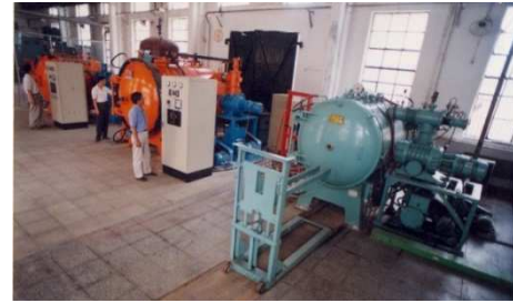
Figure 23. Pilot production line of plasma surface metallurgy plate and blade.
