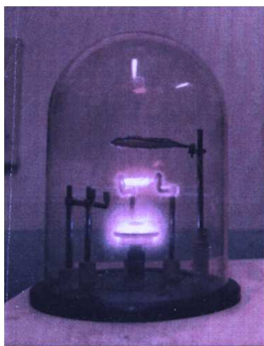
Figure 4. Double glow discharge phenomenon.
