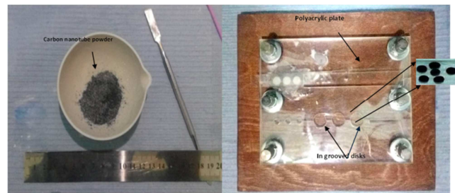
Figure 2. Concave carbon nanotubes buchydisk squeezed between syringe polypropylene and polyacrylic groove.
