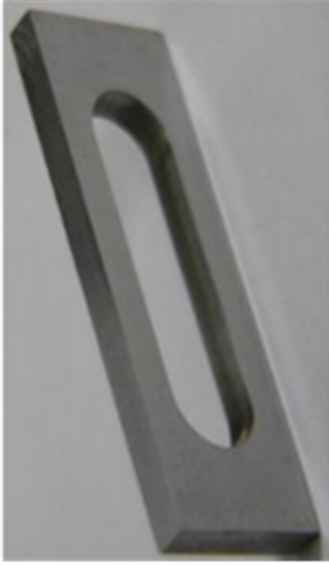
Figure 3. A photos of the small Two-bar specimen.
