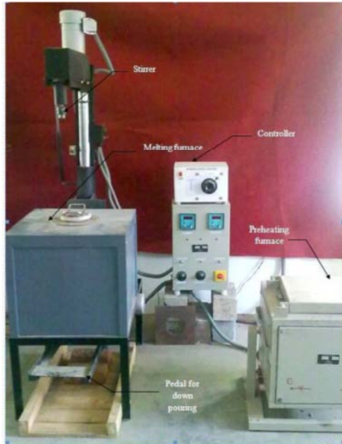
Figure 1. Stir casting setup.
