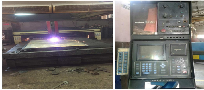
Figure 1. Plasma arc cutting machine with its control panel.
