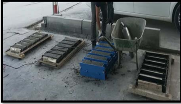
Figure 4. RCC Sample pouring and compaction.
