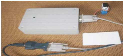
Figure 2. Intersoft RFID Demo Kit for Student's Attendance [13].
