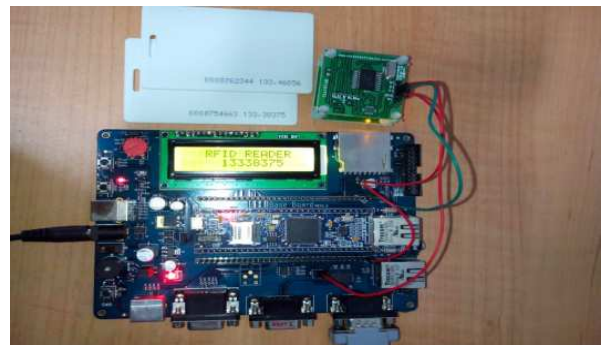
Fig 18. Photograph of RFID (125 kHz) interfaced with LPC1768
