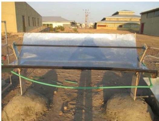
Figure 3. Installed Parabolic Solar Concentrator.
