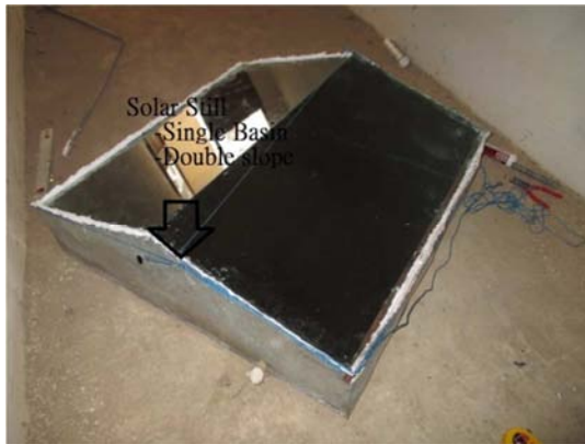
Figure 2. Manufactured single basin double slope solar still.
