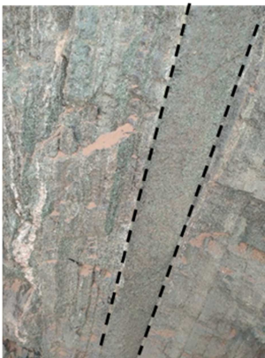
Figure 2. Discontinuity plane in the wall.
