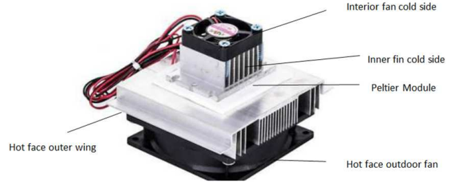
Figure 3. Thermoelectric installation composed of Peltier module.
