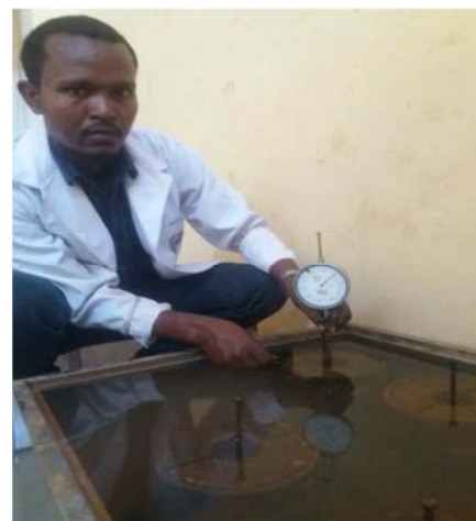
Figure 6. Measuring soaked CBR with its machine.
