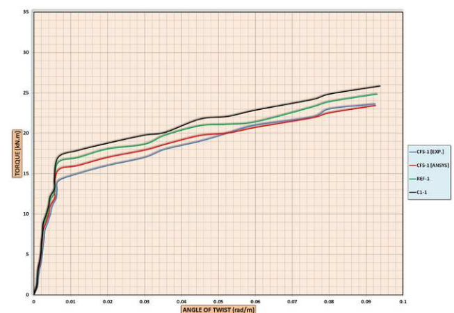
Figure (18). Effect of presence of CFRP on torque - twist behavior
