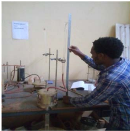
Figure 5. Falling head permeability (rate of capillary) test determination.
