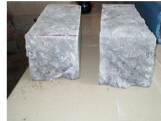
a: unreinforced cement composite beam (control).
