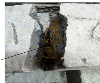
b: 1-fabric layer reinforced cement composite beam.
