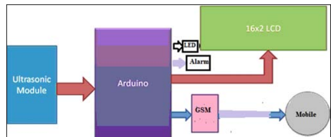
Figure 10. Flow diagram of warning device.
