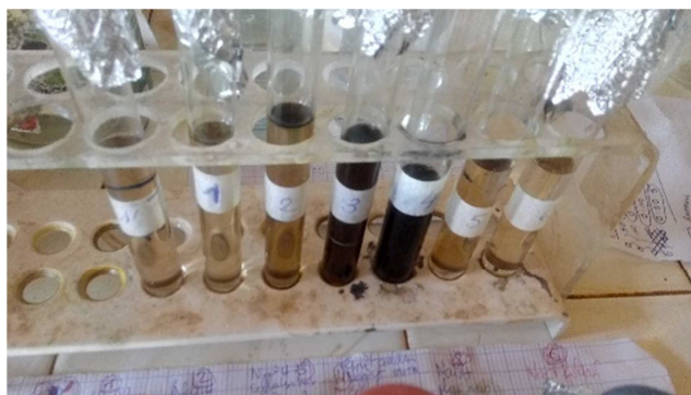
Figure 1. Colorations of the sample after concentrated 80% sulfuric acid treatment with adding 0.2ml of iodine 3.34[g/l].
