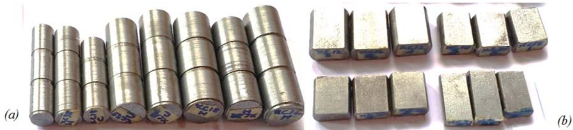
Figure 2. Samples after the first machining operations: (a) turned specimens – (b) milled specimens.
