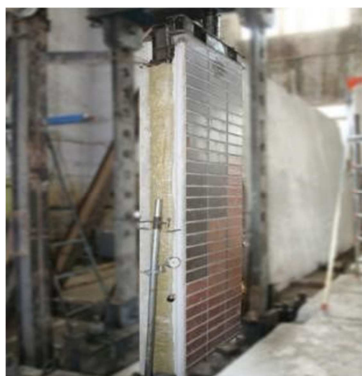
Figure 2. Fragment of a three-layer outer wall panel with composite flexible diagonal ties during shear tests.
