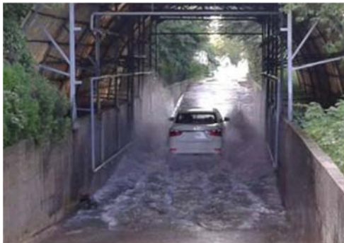
Figure 30. 15cm deep water tank wading test vehicle.
