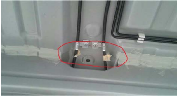
Figure 10. Leaking glue under the floor.
