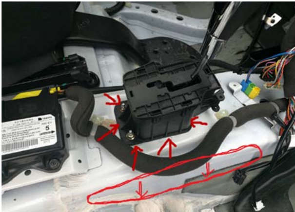
Figure 6. Water inlet on position of gear shifter.
