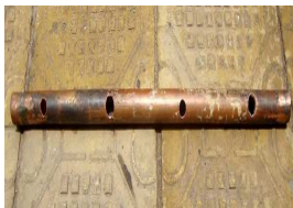
Figure 8. Header pipe under to condenser
