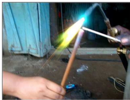
Figure 6. Brazing the block.
