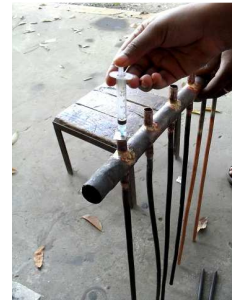
Figure 12. Injecting Acetone
